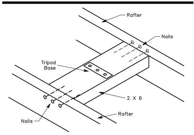
**Fig 44**—This cutaway view illustrates how the tripod tower is secured to the roof rafters. The leg to be secured to the crosspiece is placed on the outside of the roof. Another cross member is fastened to the underside of the rafters. Bolts, inserted through the roof and the two cross pieces, hold the inner cross member in place because of pressure applied. The inner crosspiece can be nailed to the rafter for added strength.
