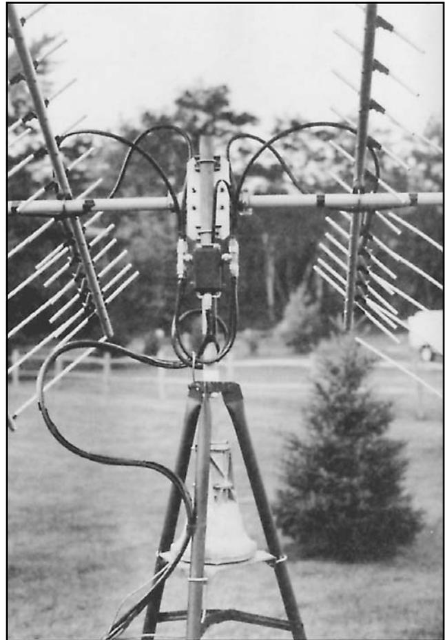
**Fig 47—Rotator loop for UHF Yagi array. The feed coax is bundled with a control cable for the polarization relay. The coax/control-cable loop is taped to the rotating mast and to the top of the tower with vinyl electric tape to allow the array to be rotated.**
