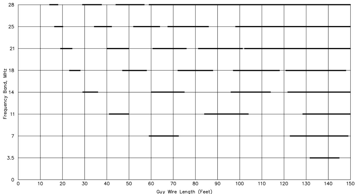
**Fig 30—The black bars indicate ungrounded guy wire lengths to avoid for the eight HF amateur bands. This chart is based on resonance within 10% of any frequency in the band. Grounded wires will exhibit resonance at odd multiples of a quarter wavelength. (By Jerry Hall, K1TD.)**
