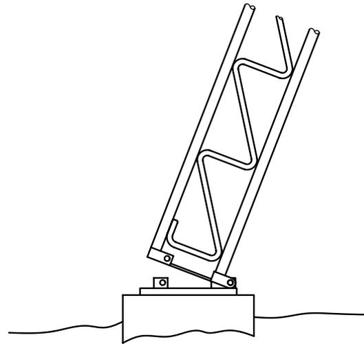
**Fig 17—Fold-over or tilting base. There are several different kinds of hinged sections permitting different types of installation. Great care should be exercised when raising or lowering a tilting tower.**
