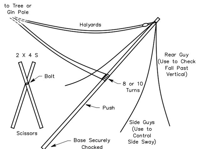
**Fig 13—Pulling on a gin line fastened slightly above the center point of the mast and on the halyards can assist in erecting a tall mast. The tensions should be just enough to keep the mast in as straight a line as possible. The “scissors” may be used to push on the under side and to serve as a rest if a pause in raising becomes necessary.**
