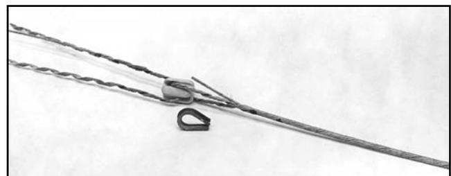
**Fig 26**—Alternative method for attaching guy wires using *dead ends*. The dead end on the right is completely assembled (the end of the guy wire extends beyond the grip for illustrative purposes). On the left, one side of the dead end is partially attached to the guy wire. In front, a thimble is used where a sharp bend might cause the guy wire or dead end to break.
