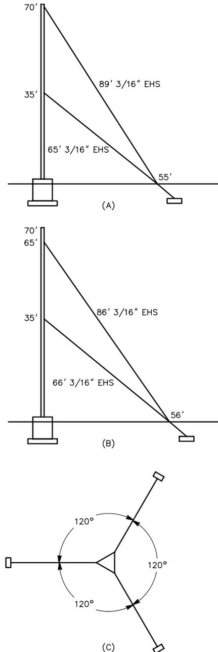
**Fig 14—The proper method of installation of a guyed tower. At A, the method recommended for most amateur installations. At B, the method shown in later Rohn catalogs. This places considerable strain on the top section of the tower when large antennas are mounted on the tower.**
