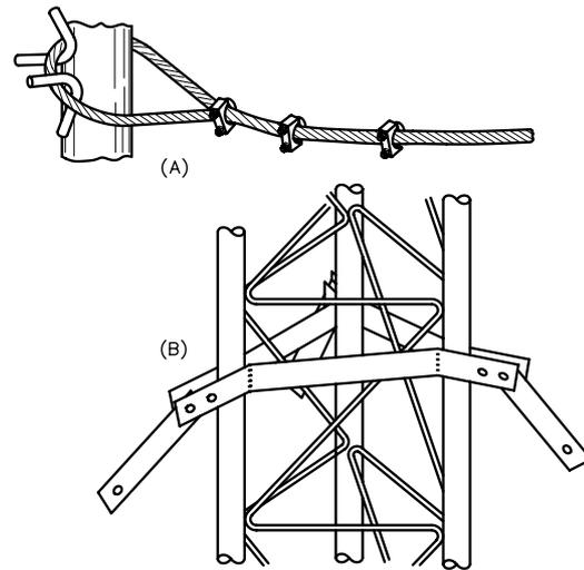
**Fig 27—Two methods of attaching guy wires to tower. See text for discussion.**
