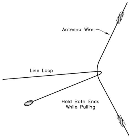
**Fig 3**—A weighted line thrown over the antenna can be used to pull the antenna to one side of overhanging obstructions, such as tree branches, as the antenna is pulled up. When the obstruction has been cleared, the line can be removed by releasing one end.
