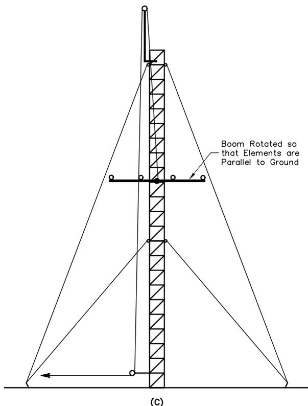
**Fig 34—Building a Yagi partway down the tower. At A, the boom is lashed temporarily to the tower and elements are added, starting at the bottom. At B, the temporary rope securing the boom to the tower is removed and the boom is rotated 90° so that the elements are vertical. At C, the boom is rotated another 90°, “weaving through” guy wires if necessary, until the elements are parallel with the ground, whereupon the boom is secured to the tower.**
