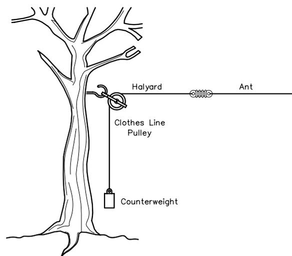
**Fig 1—A method of counter weighting to minimize antenna movement and avoid its breaking from tree movement in the wind. The antenna may be lowered without climbing the tree by removing the counterweight and tying additional rope at the bottom end of the halyard. Excess rope may be left at the counterweight for this purpose, as the knot at the lower end of the halyard will not pass through the pulley.**
