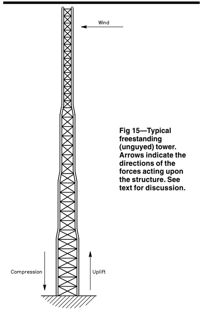
**Fig 15—Typical freestanding (unguyed) tower. Arrows indicate the directions of the forces acting upon the structure. See text for discussion.**
