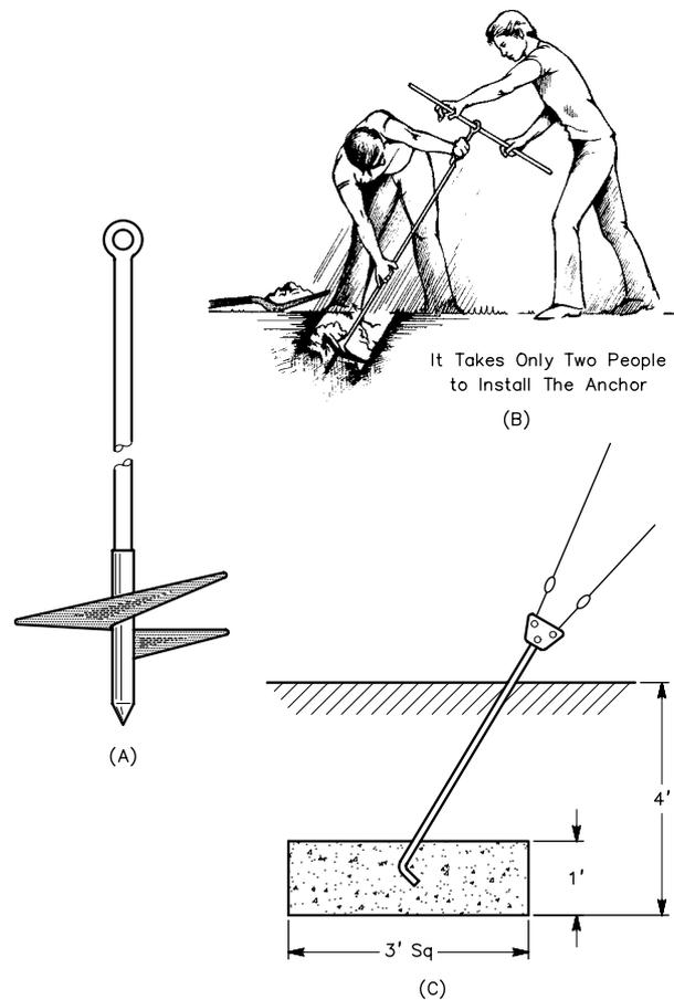
**Fig 28—Two standard types of guy anchors. The earth screw shown at A is easy to install and widely available, but may not be suitable for use in certain soils. The concrete anchor is more difficult to install properly, but it is suitable for use with a wide variety of soil conditions and will satisfy most building code requirements.**
