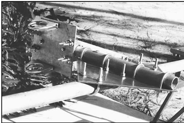
**Fig 39**—Close-up of the PVRC mount. The long pipe (horizontal in this photo) is the rotating mast. The U bolts in the vertical plate at the left are ready to accept the antenna boom. The heads of two locking pins (bolts) are visible at the midline of the boom plate. The other two pins help secure the horizontal pipe to the large steel mast plate. (The head of the bolt nearest the camera blends in with the right hand leg of the U bolt behind it.)
