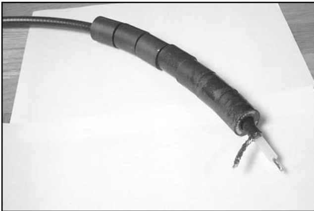
Fig 34—Choke balun made by N6BV, consisting of seven large ferrite beads strung over the jacket of a piece of RG-213 coax. This photo was taken before a layer of black electrical tape was wound over the beads to secure and waterproof the assembly on the cable.
