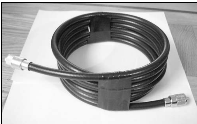
Fig 30 —An RF choke is formed by coiling the coax at the point of connection to the antenna. The inductance of the choke isolates the antenna from the remainder of the feed line. See text for details.
