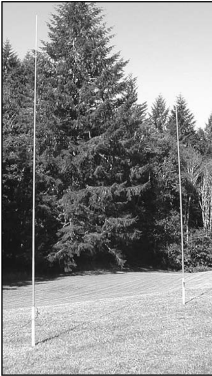
Fig 69— 2-element 20-meter phased array (Photo courtesy N7MQ).
