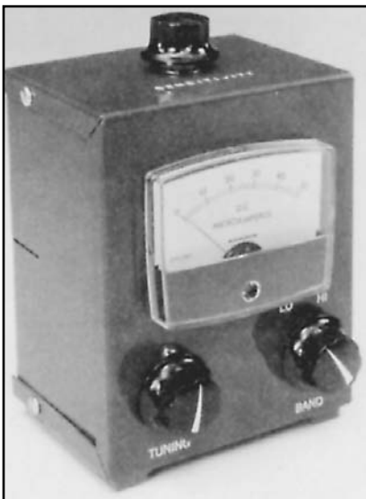
Fig 57—The RF current probe. The sensitivity control is mounted at the top of the instrument, with the tuning and band switches on the lower portion of the front panel. Frequency calibration of the tuning control was not considered necessary for the intended use of this particular instrument, but marks identifying the various amateur bands would be helpful. If the unit is provided with a calibrated dial, it can also be used as an absorption wavemeter.
