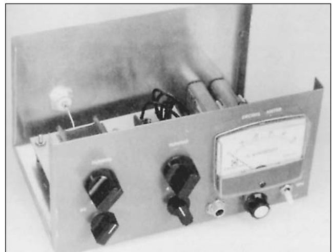
Fig 54—The linear field strength meter. The control at the upper left is for C1 and the one to the right for C2. At the lower left is the band switch, and to its right the sensitivity switch. The zero-set control for M1 is located directly below the meter.
