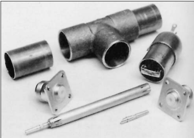
Fig 22—Major components of the line sampler. The brass T and two end sections are at the upper left in this picture. A completed probe assembly is at the right. The N connectors have their center pins removed. The pins are shown with one inserted in the left end of the inner conductor and the other lying in the right foreground.
