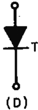
Figure 3-10D.—Tunnel diode schematic symbols.
