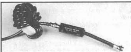
Figure 6.27—A 75-Ω high-pass filter has been installed with a common-mode choke. This combination will eliminate nearly all TVI from signals that are entering the set by way of the feed line.
