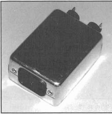
Figure 15.9—An ac-line filter at the computer power supply can reduce RF leaving through the power cord.
