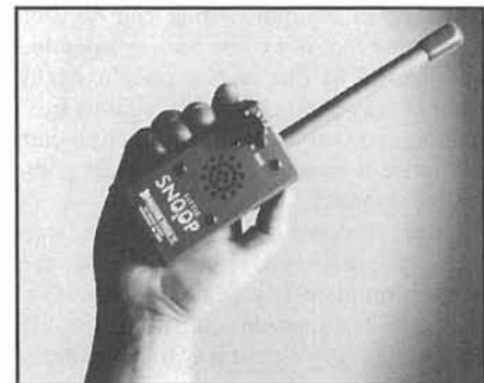
Figure 11.15 —This hand-held RF sniffer made by Micro-Tech, Inc can be used to find noise sources in or near residences. If this building is the source of RFI noise, the noise will be very strong near the power meter. A hand-held sniffer should never be used near high-tension lines and should never be allowed to contact any source of ac-line voltage in the home.
