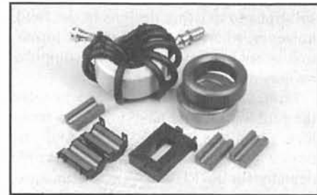
Figure 15.7—Several different ferrite cores that can be used to help cure computer RFI.
