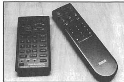
Figure 8.13—Typical VCR wireless remote controls operate with infrared, rather than RF. That’s a blessing.
