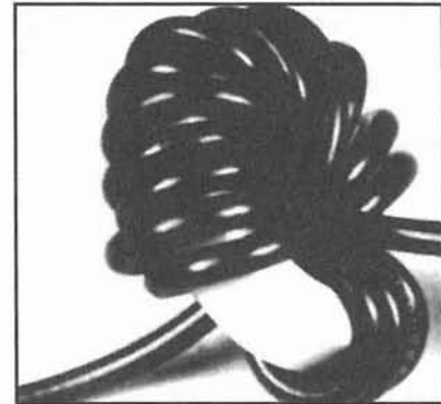
Figure B—A common-mode choke is the first line of defense against CATVI! This choke can be easily made with a few turns of wire onto an F(T)-240-43 or -75 ferrite core. See the EMC Fundamentals chapter for more information.
