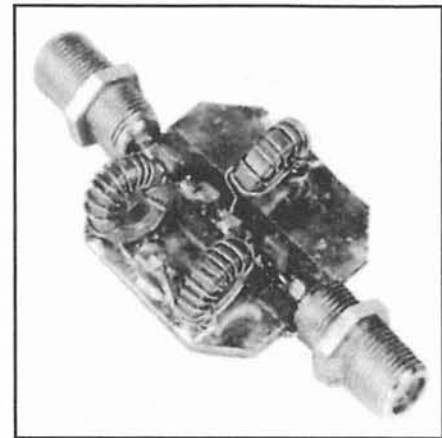
Figure 6.35—Photo showing construction of the 75- \Omega unbalanced filter. Double-sided \frac{1}{16} -inch FR-4 epoxy-glass PC board is used as a base for the filter components. A section of copper on the top is stripped away on both sides of center to approximate a 75- \Omega microstrip line about \frac{3}{32} -inch wide. Both sides of the top copper foil (at the edges) are connected to the ground plane foil underneath.
