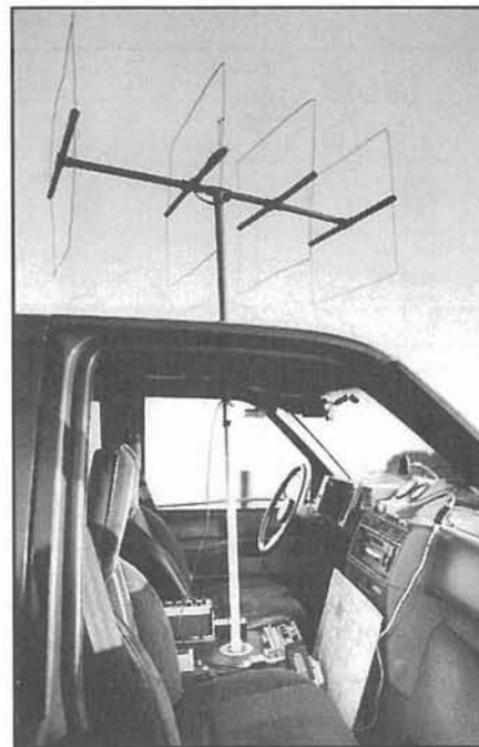
Figure 4.10— K0OV uses this mobile setup for RDF on several bands, with separate antennas for each band that mate with a common lower mast section, pointer and 360° indicator. Antenna shown is a heavy gauge wire quad for 2 m.
