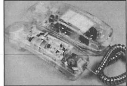
Figure 9.1 —This telephone is transparent to light so we can see right through it. If we could see what RF sees, most telephones would look like this!
