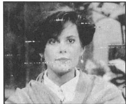
Picture 7: Electrical Interference—low noise
