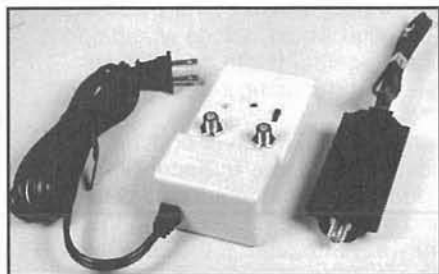
Figure 6.7—A TV preamp. These devices are not necessary in strong signal areas, and in many cases are the cause of TVI.
