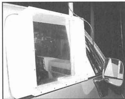
Figure 4.16—A window box allows the navigator to turn a mast mounted antenna with ease while remaining dry and warm. No holes in the vehicle are needed with a properly designed window box.
