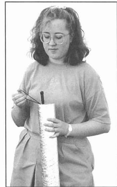
Figure 4.21—The air attenuator for a VHF hand-held in use. Suspend the radio by the wrist strap or a string inside the tube.
