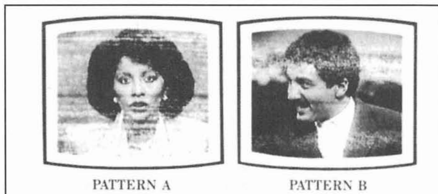
Figure 6.15—Two examples of TVs experiencing electrical noise.
