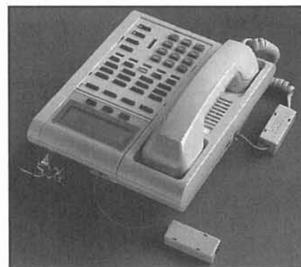
Figure 9.14 —To cure interference to the telephones at ARRL Headquarters, it was necessary to install a phone filter on the telephone line, a separate filter on the handset cord and a home-brew common-mode choke on the dc power supply lead. This phone now works at W1AW when the bulletins are running on all seven bands!
