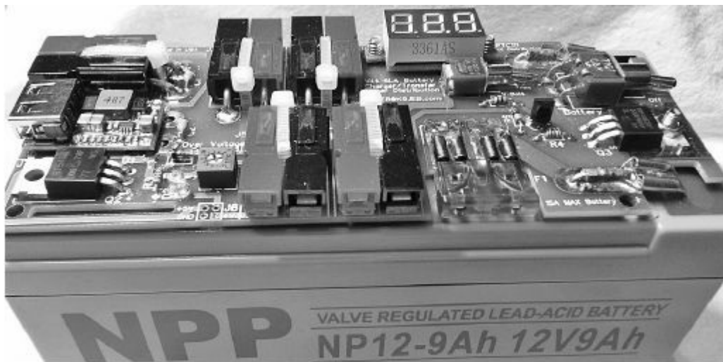
Figure 7.67 — The charging circuit shown mounted directly on a 9 Ah SLA battery. Note the USB charging module mounted next to J1 at the left-hand side of the board.
