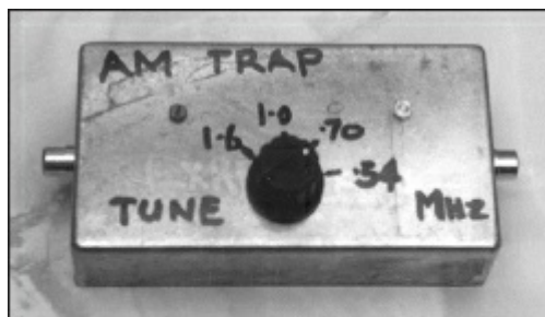
Figure 10.69 — The wave trap can be roughly calibrated to indicate the frequency to which it is tuned.
