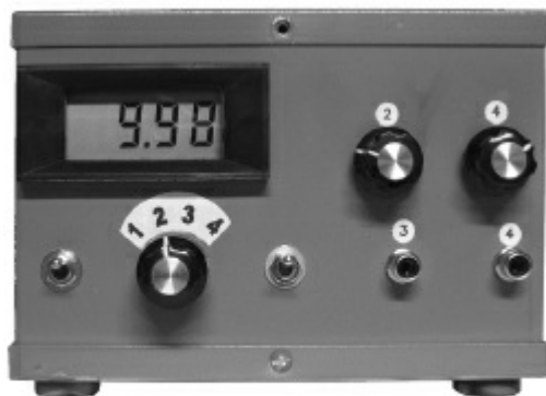
Figure 7.55 — The front panel of the four-output switching supply.
