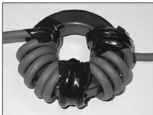
Figure 5.50 — A ferrite choke consisting of multiple turns of cable wound on a 2.4-in. OD \times 1.4-in. ID \times 0.5-in. toroid core.
