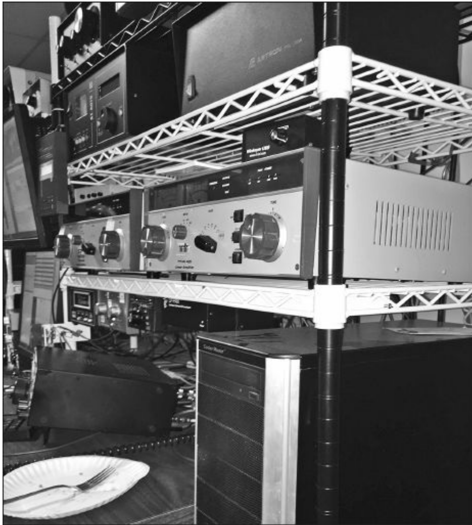
Figure 24.16 — Taking advantage of a good opportunity, N0NI adapted this set of metal wire shelving to hold his equipment. The wire shelves also act as an RF ground plane and provide ventilation. [Bob Lee, W0GXA, photo]
