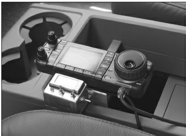
Figure 24.23 — In this mobile installation, the transceiver control head is mounted in the center console, next to a box with switches for adjusting the antenna.
