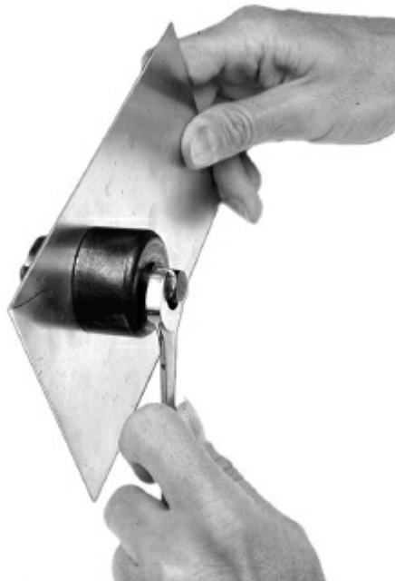
Figure 23.3 — A socket punch is used to punch a clean, round hole in sheet metal.
