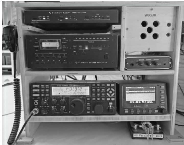
Figure 24.14 — This portable 500 W HF station was constructed by W6GJB and K9YC for portable operation during the California QSO Party. [Jim Brown, K9YC, photo]
