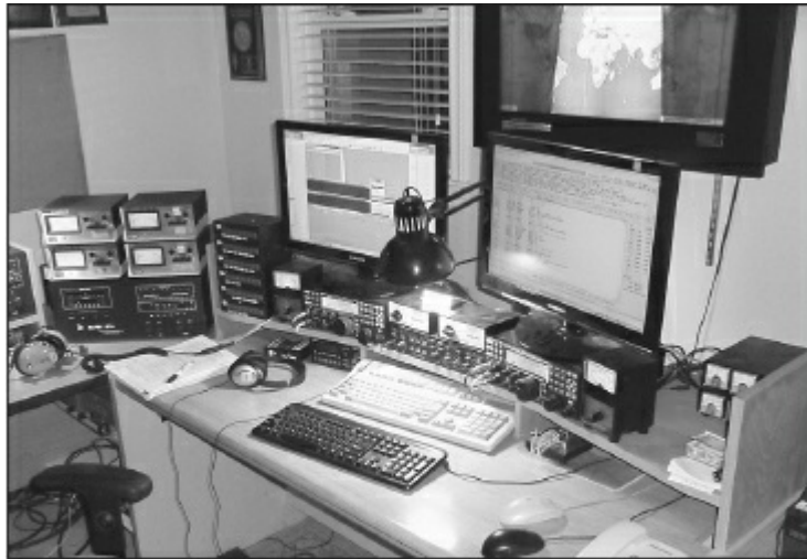
Figure 24.3 — Spreading out horizontally, John Sluymmer, VE3EJ, has arranged his effective contest and DXing station to keep all of the controls at the same level for easy adjustment. [John Sluymmer, VE3EJ, photo]
