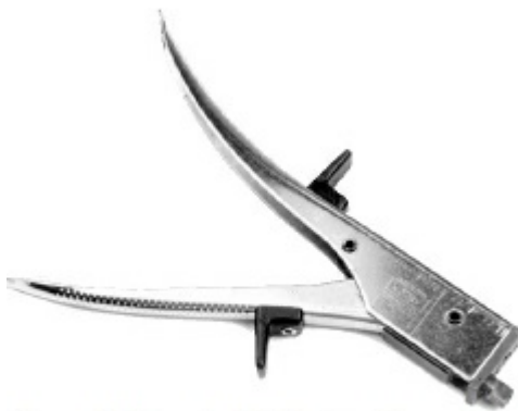
Figure 23.1 — A nibbling tool is used to remove small sections of sheet metal.
