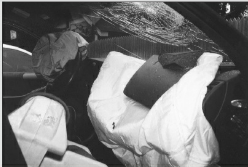
Figure 24.B — Airbag deployment following a minor collision caused significant disruption inside the passenger compartment.
