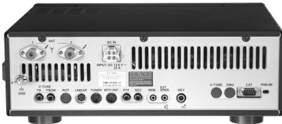
Figure 24.18 — The back of this Yaesu FT-950 transceiver shows some of the many types of connectors encountered in the amateur station. Note that this variety is found on a single piece of equipment.
