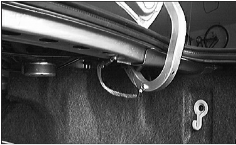
Figure 24.29 — Bonding vehicles parts — in this case, the trunk lid to the main body — can help reduce interference.
