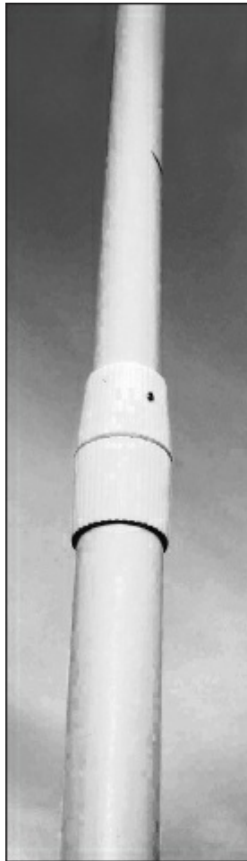
Figure 24.33 — Close-up of a telescoping mast. Sections slide together and are secured by twisting a locking mechanism.
