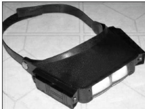
Figure 23.6 — A magnifying visor is great for close-up work on a circuit board. These headsets are often available for less than $10 at hamfests and some even come with superbright LEDs mounted on the side to illuminate the components being soldered.
