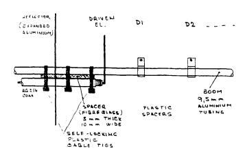
In fact, this type of mounting of the elements is very suitable for optimizing the spacings of individual elements. However, I would not recommend trying any adjustments unless you really know what you are doing and have some measuring equipment and reasonable space for experiments.
