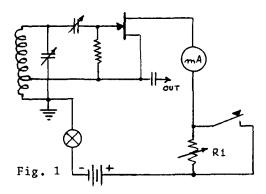
The oscillator in Fig. 1 is shown for clarity -- any good oscillator circuit may be used. Oscillator feedback and R1 are adjusted for minimum change in bias current with keying, consistent of course with the oscillator starting and stopping. Let me borrow a term from the good old days and call it "keep-alive keying." - A. H. Mehner. W7HP, 611 South Tonopah Drive, Las Vegas, NV 89106.
