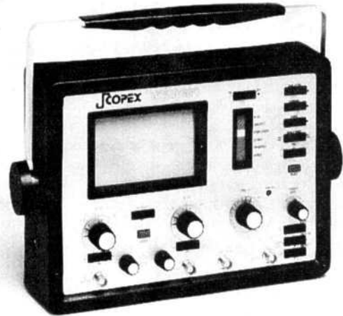
Fig. 12 Commercially available digital storage oscilloscope with 10 cm × 6 cm dyed-phasechange liquid-crystal display
