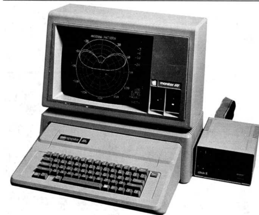
An antenna radiation pattern, calculated by Annie, is displayed on an Apple IIe system.
