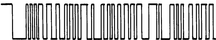
Fig 5—The output of PN generator U7, at pin 2. The scanning rate is 5 \mu s/div.
