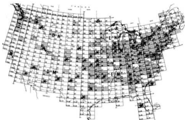
Fig 1—Total aurora activity on 144 MHz. Shaded grid squares represent the location of at least one reported 144-MHz aurora contact during Feb 7-9. Logs were received from the squares marked with an asterisk.
