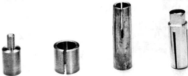
Fig 2—A threaded center pin adaptor, an expendable split sleeve, a female connector and one adaptor. The female connector is threaded at 80 tpi. These are expandable and no taper point is present at the male pin's point of entry. The male pin should be slightly tapered at the point to facilitate entry.
