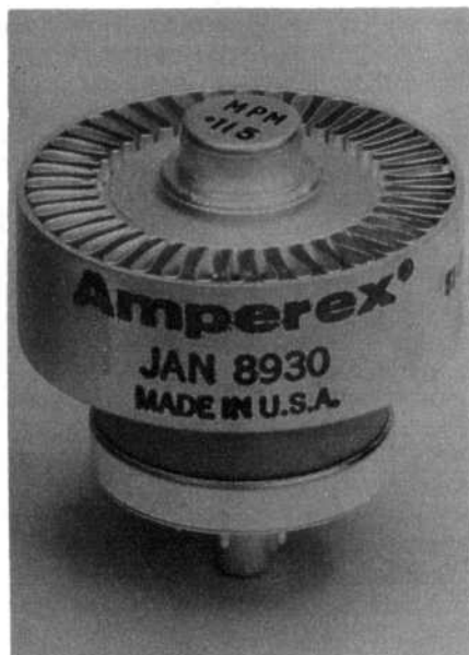
Fig 2—Similar to the 4CX250R, the 8930 is a premier tube for use at 432 MHz. Operating conditions for an 8930 in class-AB amplifier service are: anode voltage—2.5 k, screen voltage—400, plate current—250 mA, output power—300 W. See text.
