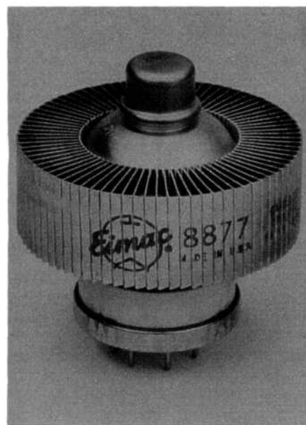
Fig 4—The 8877 is one of the more popular tubes in amateur service. Its frequency limitations are discussed in the text. Operating conditions for an 8877 in class-AB service at 220 MHz are: anode voltage—2.5 k, anode current—1 A, driving power—57 W, output power—1.52 kW.
