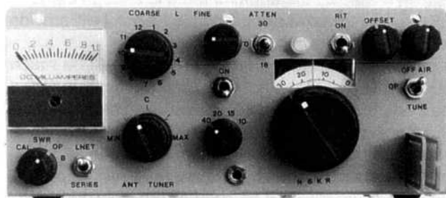
Fig 14—This view of the transceiver shows the front panel controls and labeling. The front panel is only 3 by 7 inches, so layout is critical (see text).
