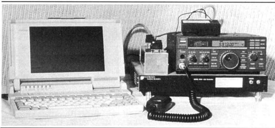
Fig 1—Low-cost HF ALE radio system.
