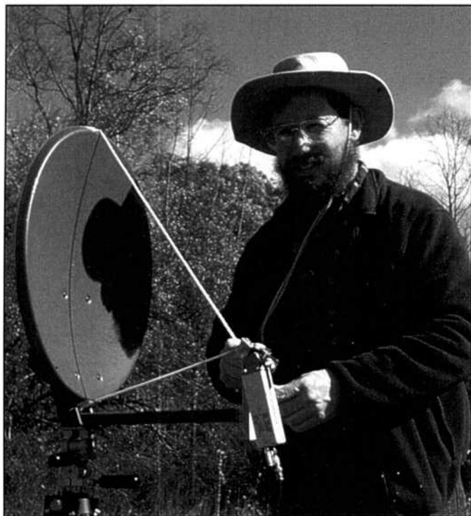
Fig 4—Locating feed point for offset dish using calculated string lengths.
