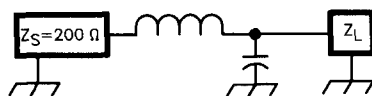
Fig 2—An L-network operating at 3.5 MHz, with a Mathcad graph that shows the matching range of the network.
