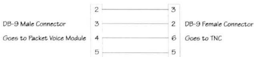
Fig 5—Pin assignments for serial connector.
