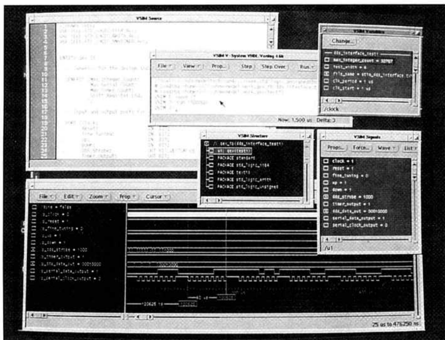
Fig 4—A VHDL simulation using the Model Technology simulator. The windows open in the photo are used to display (clockwise, from upper left-and corner) the VHDL source code, control functions, variables, signals, a waveform-trace window for I/O signals and (center window) overall design structure.
