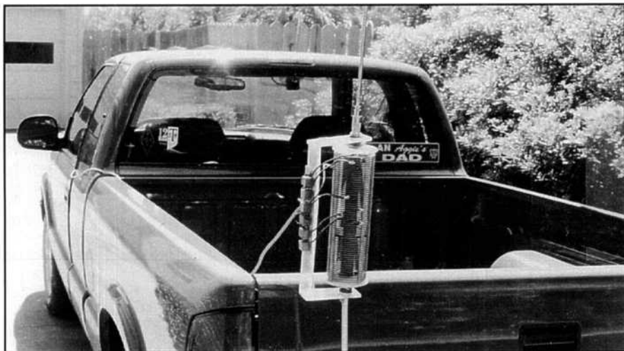
The coil and switch assembly mounted on the author's truck.
