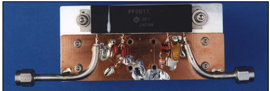
Fig 1—A microwave amplifier with complete topside foil—oscillates.
