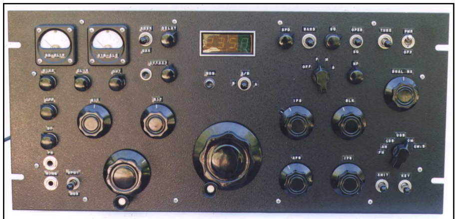
Fig 3—Front panel of the basic 40 to 39-MHz transceiver. Four of the operating features are enabled by means not apparent in the photo. The A RIT, B RIT, BLANKER , and DUAL RX knobs are all attached to potentiometers with ganged push-pull switches. Pulling the knob out actuates the function.
