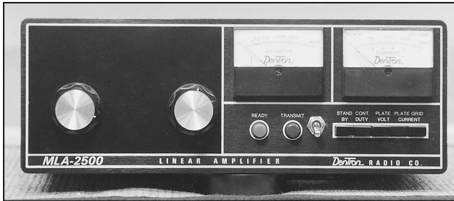
Fig 6—The front panel of the converted MLA2500. The left side has been covered with a thin, black aluminum plate. Note the new power switch between the TRANSMIT light and the STAND BY switch.
