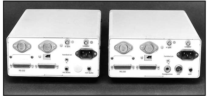
Fig 3—Rear view of the remote (left) and control (right) 10-GHz transceivers.
