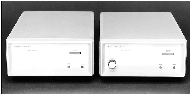
Fig 2—Front view of the remote (left) and control (right) 10-GHz transceivers.
