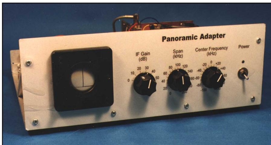
Fig 13—Front panel showing controls and display.
