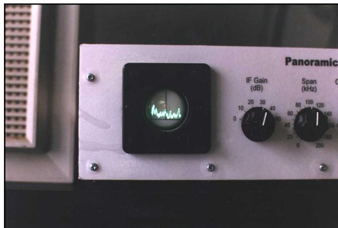
Fig 14—A close up of the CRT shows signals on 20 meters. Center frequency is 14.2 MHz, span is 100 kHz.
