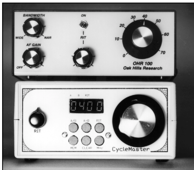
Fig A—Front Panel of the CycleMaster. Notice that the seven-segment displays are inverted, so that the decimal point can serve as an A/B VFO and RIT indicator.
