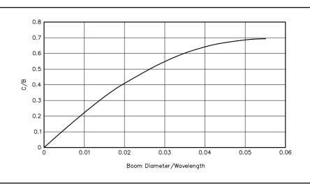
Fig 1—Plot of G3SEK's formula for boom correction.
