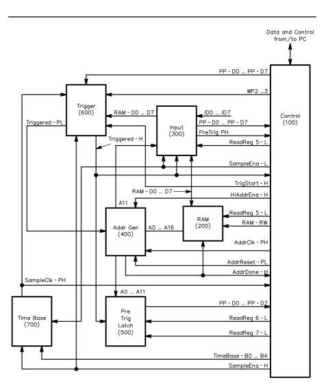
Fig 1—Logic Analyzer block diagram.
