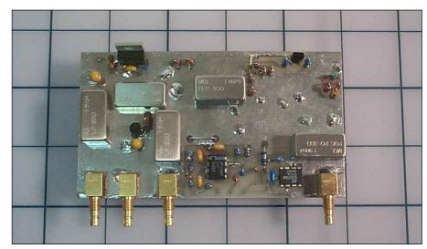
Fig 9—The PC boards are constructed with the through-hole components mounted to the top of the board. This is a view of the Mixer board component side.
