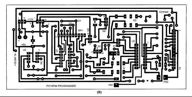
Fig 6—(A) PIC controller etching pattern, full size 3.87×6.07 inches. (B) PIC programmer etching pattern, full size 2.92×6.21 inches.
