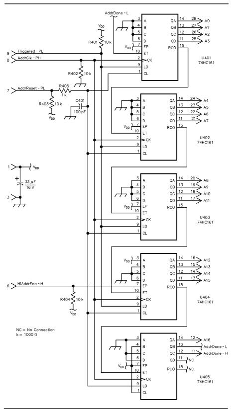
Fig 2—Address Generator schematic diagram.
