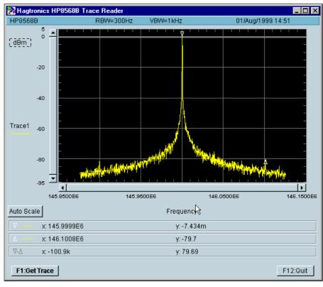
Fig 8—The close-in spurious performance of the source shows a reference rejection of -80 dBc. The span for this display is  $\pm 125$  kHz from the carrier.
