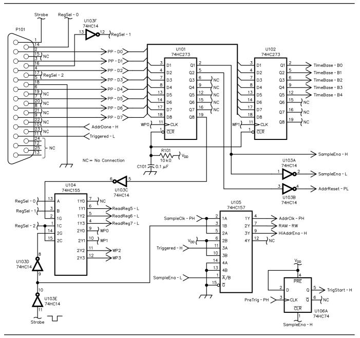
Fig 3—Control circuit schematic diagram.
