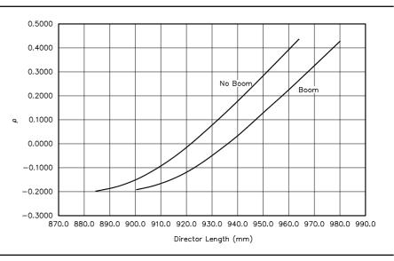
Fig 2—Data for frequency 144.2 MHz, *B* = 32.0 mm, *d* = 6.35 mm.
