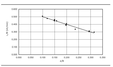
Fig 5—Dependence of inductance L on B and d.
