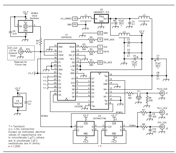
Fig 2—The NCO circuit is used to derive the master-clock references for the rest of the source. The NCO-driven, 10.7-MHz output is used as a super-fine adjustable reference for the PLL 0 board. PLL 1 and the PIC microprocessor are driven by fixed 10-MHz clocks. Unless otherwise specified, use 1/4 W, 5%-tolerance carbon composition or film resistors. All capacitors are 50-V X7R ceramics unless otherwise noted.
