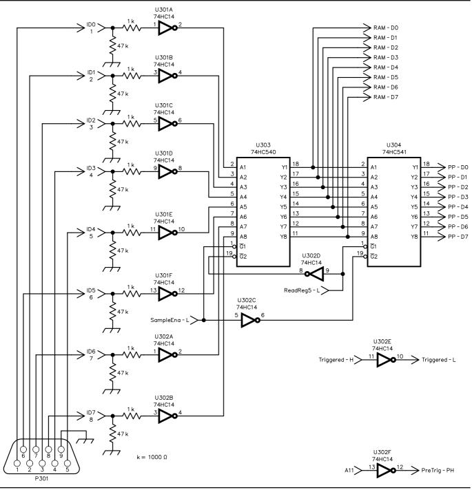
Fig 4—Input circuit schematic diagram.
