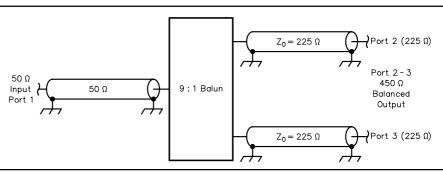
Fig 4—Modeling a 450- $\Omega$  balanced line as two 225- $\Omega$  coaxial lines with ARD's three-port model.
