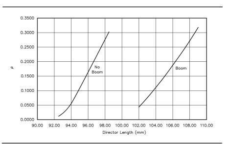
Fig 4—Data for frequency 1296.2 MHz, *B* = 16.2 mm, *d* = 4.76 mm.
