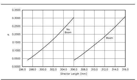
Fig 3—Data for frequency 432.2 MHz, B = 20.2 mm, d = 4.76 mm.
