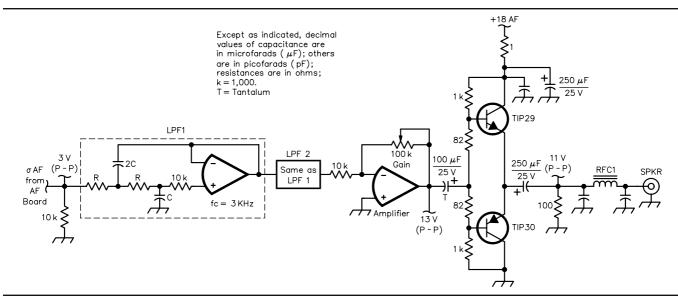
Fig 8—AF-output-module schematic diagram. For general notes on the schematics, refer to the caption for Fig 3. The 1- $\Omega$  resistor in the +18-V supply line to the output stage is a shunt for current metering during tests. A DMM set to the millivolt range will read out in milliamps directly. These 1- $\Omega$  shunts are also included at many other points in the radio where a current measurement is required. The complementary-output transistors are available at Hosfelt.
