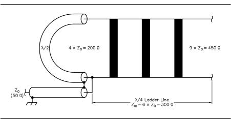
Fig 3—A 9:1 balun using  $\lambda/2$  of coax and a 300- $\Omega \lambda/4$  matching section.
