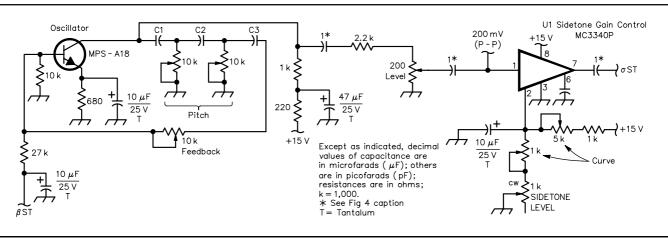
Fig 7—Sidetone-oscillator schematic diagram. For general notes on the schematics, refer to the caption for Fig 3. C1-C3—Polypropylene capacitor, 47 nF. U1—MC3340P. See caption for Fig 4. Panasonic #ECQ-P1H473GZ, Digi-Key #P3473.
