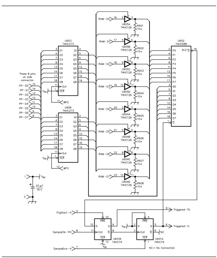
Fig 8—Trigger circuit schematic diagram.
