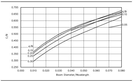
Fig 6—Boom corrections *C*/*B* for elements of length 0.42  $\lambda$  and for various *d*/*B* values.
