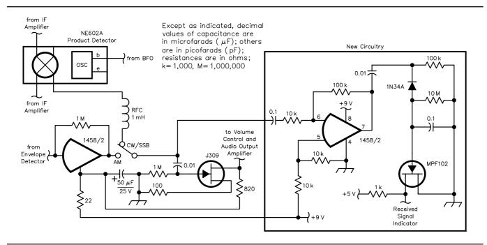
Fig 3—Received-signal indicator circuit.
