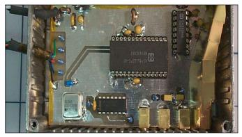
Fig 11—All major circuit blocks in the source are designed to be mounted in low-cost, die-cast enclosures from Jameco. Here is a view of a completed NCO board with some added shielding (on the right side) around the 10.7-MHz filter to reduce any clock feed-through to the 10.7 MHz PLL reference signal.
