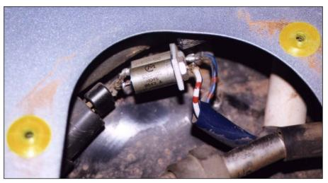
Fig 2—Filter cons installed on bracket.
