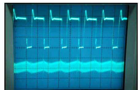
Fig 7—Low-power tests of the converter. At left, the setup for the test. Above, the waveforms of the inductor input voltage and the output voltage ripple. The horizontal axis is 2 \mu s per division. The vertical axis is 10 V per division for the upper trace and 0.2 V per division for the lower trace.
