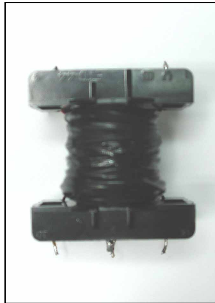
Fig 6—Construction of the center-tapped secondary coil. Two #18 AWG coils are connected in series.
