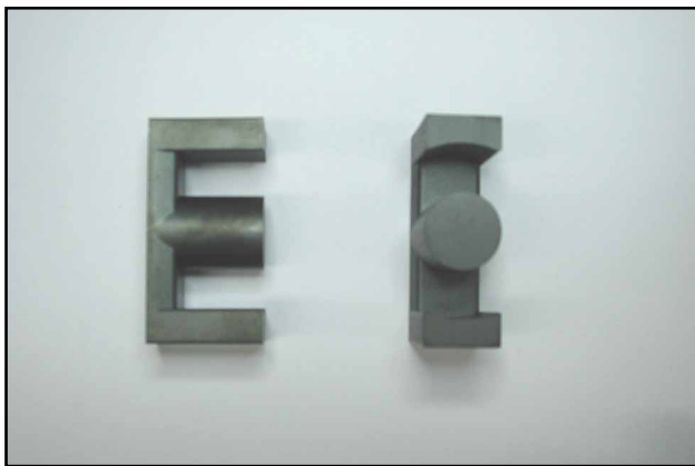
Fig 3—The ETD44 can isolate 500 W at a switching frequency of 100 kHz. The round central arm of the core improves efficiency. Each piece of the core measures 4.4×1.5×2.25 cm.
