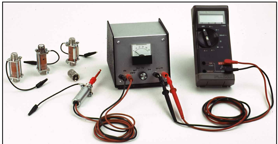
Fig 23—The meter unit with RF probes and a DVM connected to the OUTPUT jacks.
