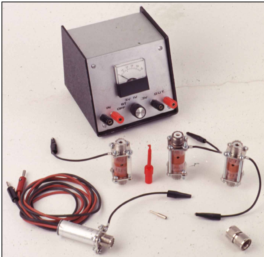
Fig 1—The RF voltmeter with meter unit, RF probe and voltage multipliers.
