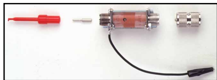
Fig 10—A view showing the 10× multiplier with grabber, pin tip and a male UHF coupler that connects the multiplier to the RF probe.
