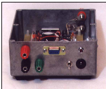
Fig 10 —The power-supply end. The wall-wart-input connector, LED and power switch are on the right. The binding posts on the left are for the +5 V reference-voltage output.
