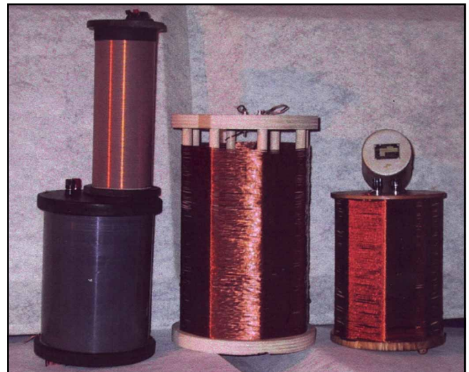
Fig 5—A group of 136-kHz big coils realized for high quality factor ( Q ).
