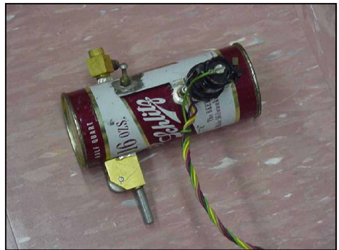
Fig 4—A side view of the beer-can polaplexer. Notice that the receiving antenna (crystal and sliding short) are about \lambda_c/4 from the closed end of the can, and the klystron and transmitting antenna are about 3\lambda_c/4 from the closed end. Judging by the label, I must have removed the bottom of the beer can rather than the top! (This can predates pull-tabs.)
