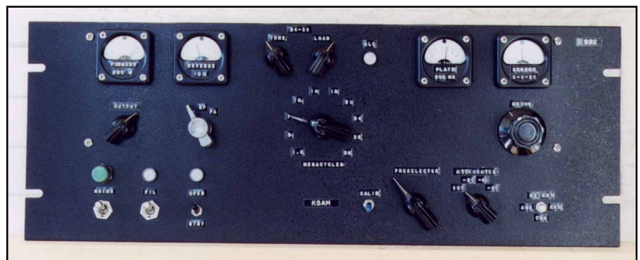
Fig 2—Front panel. Rather than trying to achieve uniformity in knob style, several different styles are used deliberately; this helps the operator find the correct knob very quickly. For consistency and additional convenience, the same style choices are also used on the other front-end sections for corresponding controls.
