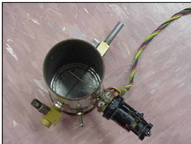
Fig 3—An end view of the beer-can polaplexer, showing the 726 klystron at 4 o'clock, the local oscillator injection screw at 6 o'clock, the crystal mount and BNC IF output at 7 o'clock and the sliding coax shorted stub at 1 o'clock.
