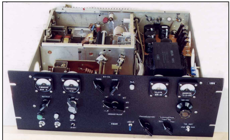
Fig 1—HF front-end section for the K5AM homebrew transceiver. The PA tank compartment is at the left rear, with its shield cover and exhaust fan removed. The 8072 conduction-cooled tetrode is clamped inside the large block. The 160 and 80-meter toroids are at the left of the PA compartment. The long “bread-slicer” capacitor is for tuning the 24-30 MHz range. (Photos by Lisa Mandelkern)
