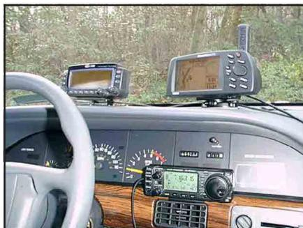
**Fig 1—Charles Richards, W4HFZ's mobile APRS satellite capability (also includes HF). With an APRS satellite, he can send and receive brief text messages anywhere on the planet a few times a day.**
