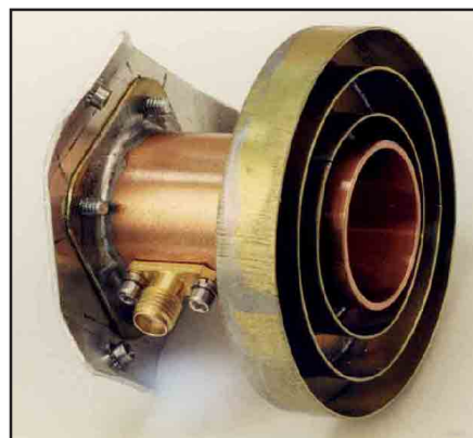
Fig 1—Homebrew Chaparral feed made out of a copper pipe coupling and brass sheet stock.
