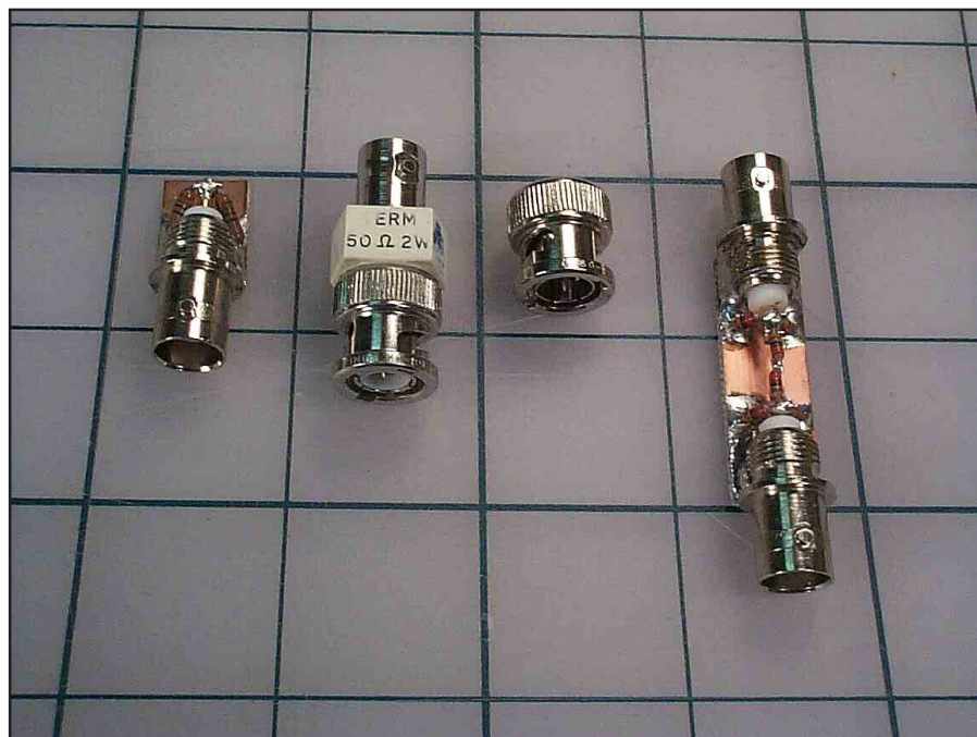
Fig 8 —The half-homemade, half-purchased calibration kit for the network analyzer consists of (left to right): a 1.5:1 (75- \Omega ) mismatch standard, 50- \Omega termination, shorting BNC end cap used for the short standard (the open standard just leaves the input port open) and lastly the 20-dB attenuation standard. I built the mismatch load and attenuator out of \frac{1}{4} -W metal-film resistors with the leads trimmed as short as possible. This arrangement gave more than adequate results at 250 MHz. 1206 SMT resistors could have also been used with slightly less physical robustness.
