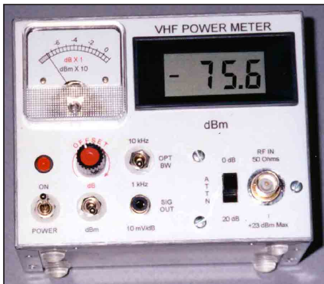
Fig 1 —The advanced VHF power meter includes a digital panel meter for accurate, high-resolution power readings plus an analog meter for trend information. The instrument bottoms out around -76 dBm but calibration very good above -70 dBm.
