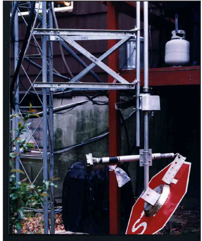
Fig 4 —The complete flyswatter assembly mounted at the bottom of a tower for tests.
