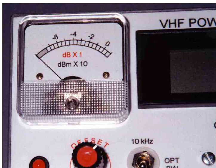
Fig 8—The original 0-1 mA meter scale has been replaced with an eye-catching and functional power-meter scale. The replacement scale was made using a drawing program and an inkjet printer.
