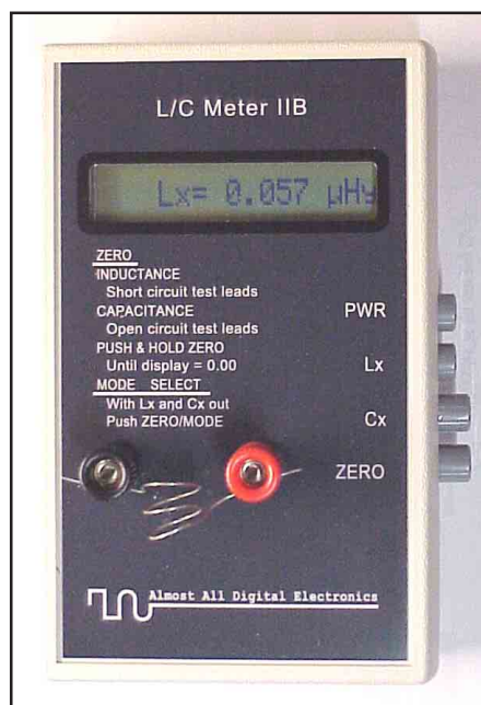
Fig 1—The L/C Meter II B from Almost All Digital Electronics (AADE) can measure small value inductors and capacitors to a fraction of a nanohenry or a picofarad.
