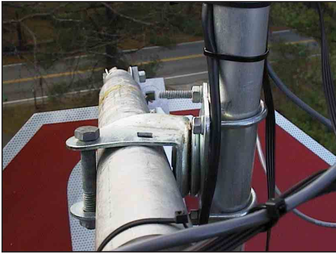
Fig 5 —A close-up view from the mast end of the actuator. A heavy-duty, flange-mounted swivel caster serves as a mount and bearing for the actuator once the caster wheel is removed. The flange is secured to the mast by two U bolts.
