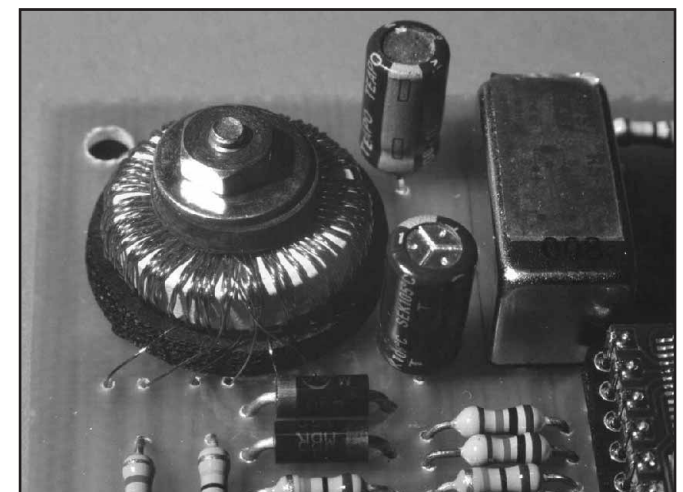
Fig 31—The toroid for the dc-dc converter was mounted using a bolt and foam rubber washers.
