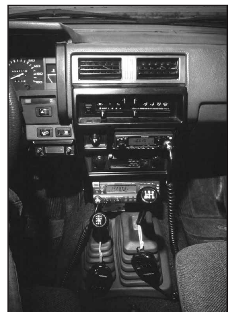
Fig 40—The author's mobile installation. Notice the microphones hung from wire loops on the gear-shift levers.
