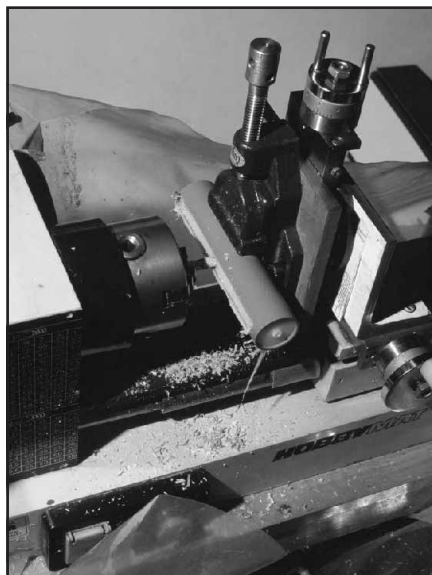
Fig 19—The lathe milling slots in the PVC tube. The quality is rough, but adequate.
