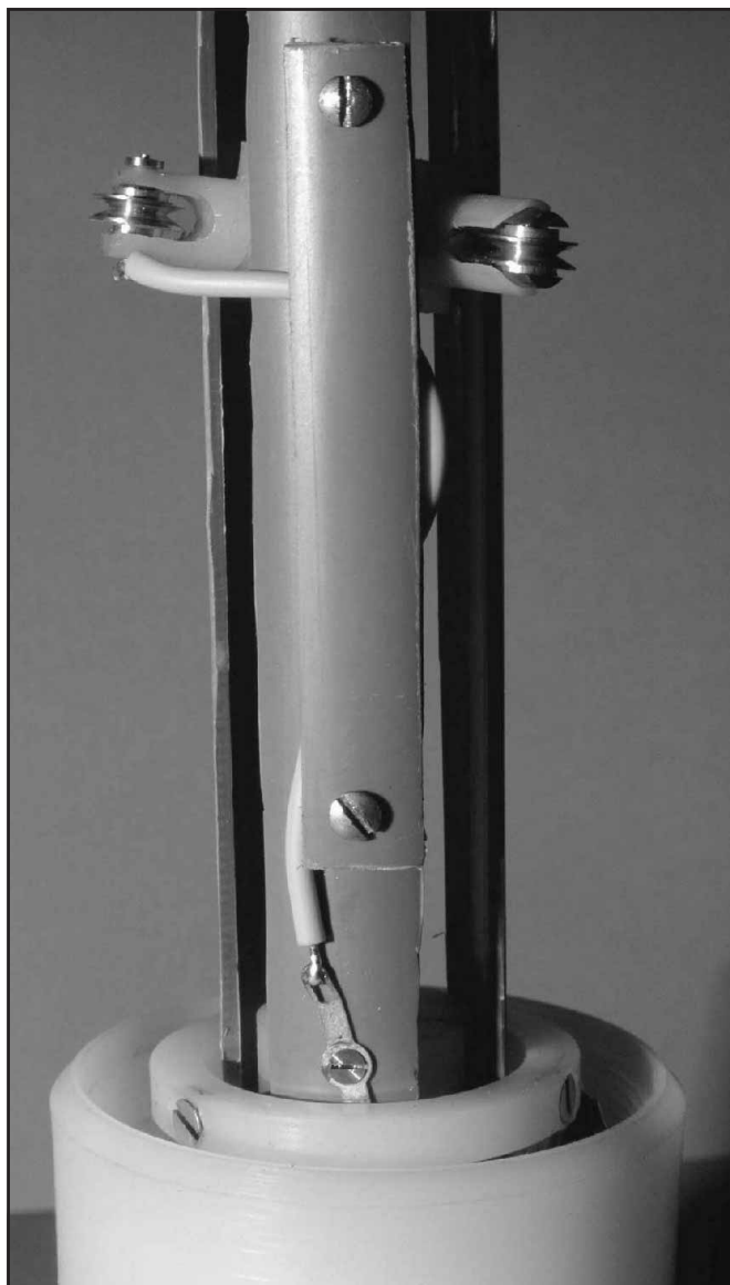
Fig 24—(left) A view of the flexible-wire routing. The text explains that this wire was later replaced with RG-174. Fig 25—(above) The complete assembly (except for the wire guide) installed in the base cup.
