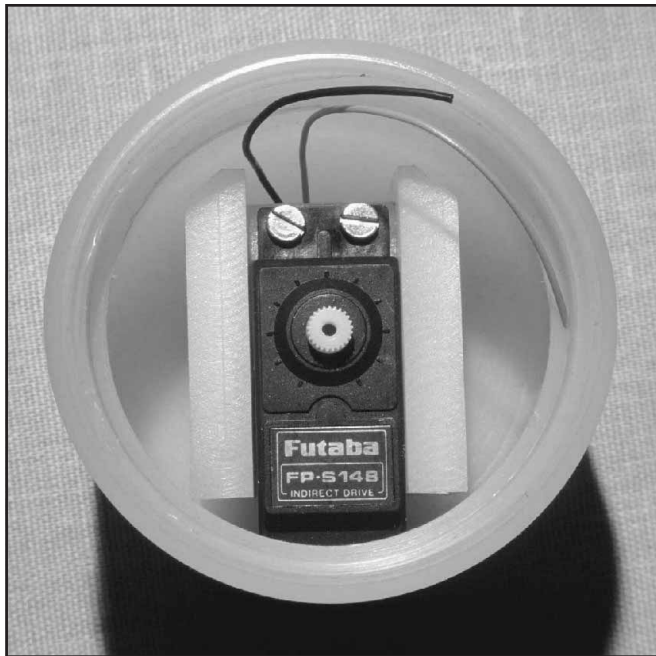
Fig 13—The servo with its mounting plates test-fitted in the base cup. Notice that one edge of each plate is chamfered.
