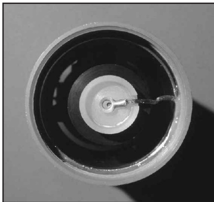
Fig 26—The loading coil assembly has been installed. This was done only for the photo, which shows how the top lead of the coil runs through a slot in the centering cup.
