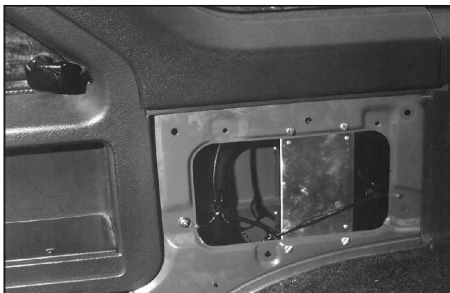
Fig 39—The controller installed under a trim panel in the author's Nissan.
