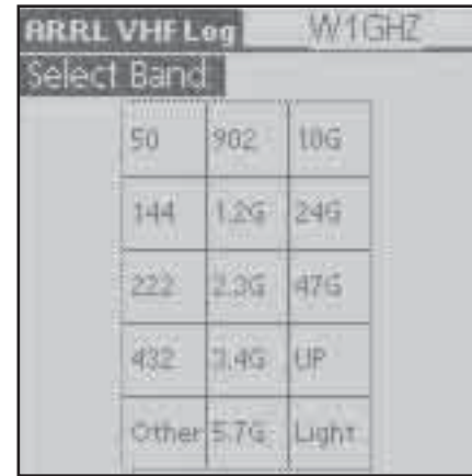
Fig 4—A single stylus tap can enter bands up through 47 GHz. Higher bands require a text entry.
