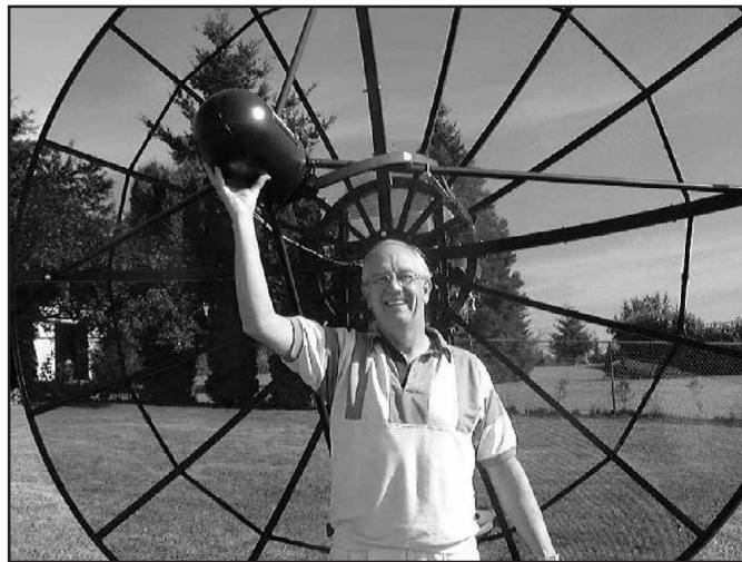
Fig 6—W7SZ with his dish antenna used on 10 GHz. The microwave equipment is mounted at the focus of the antenna. Equipment for 10 GHz is similar to that used by W7LHL except that the transmitter power amplifier uses a TWT (traveling-wave tube).
