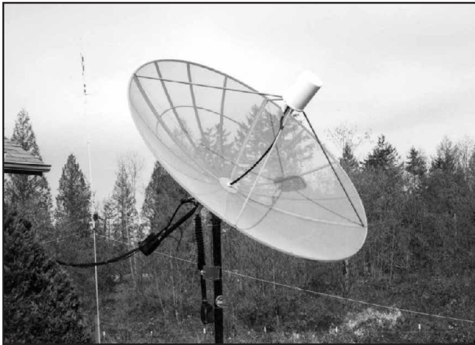
Fig 4—The 10-foot parabolic-dish antenna used for both 1296 MHz and 10 GHz by W7LHL. This is a surplus TVRO antenna. The RF equipment is mounted at the center feedpoint.
