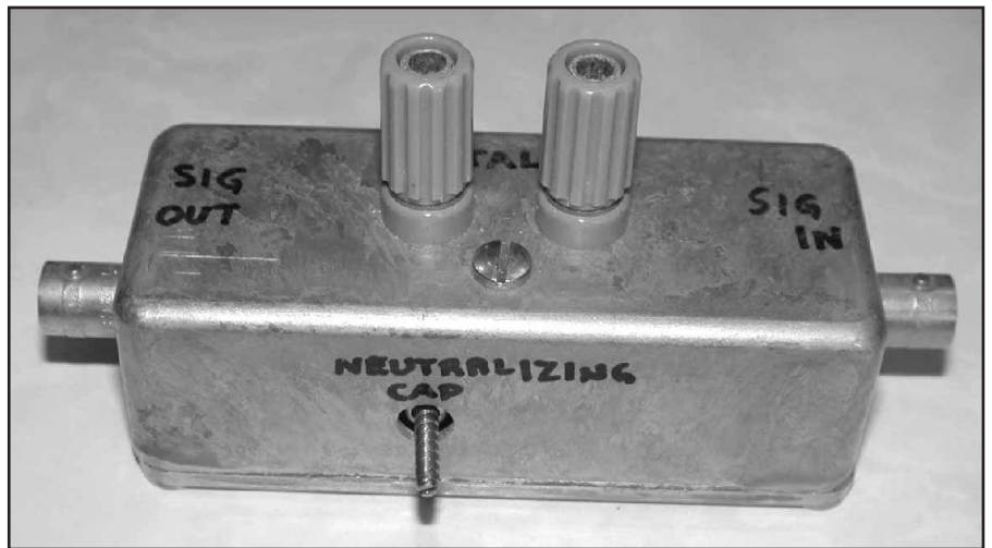
Fig 7—Outside view of crystal measuring test fixture.
