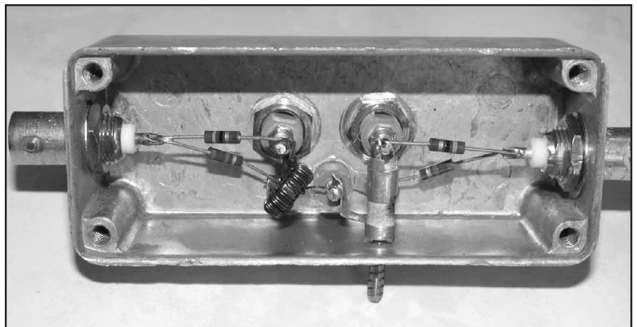
Fig 8—Inside view of crystal measuring test fixture.
