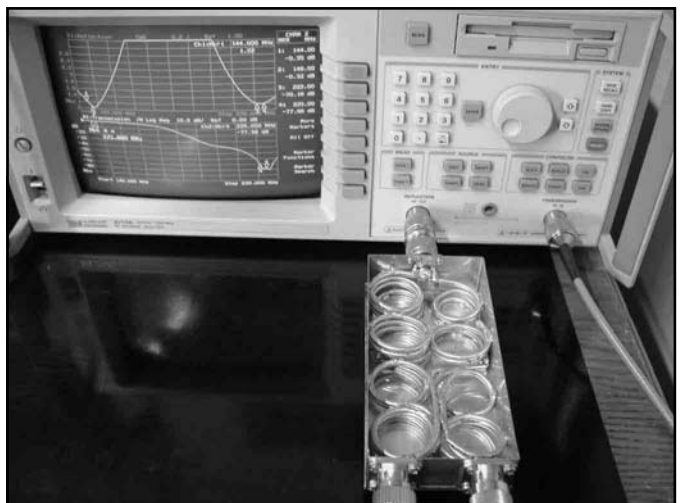
Fig 7—The 145 MHz section under measurement.
