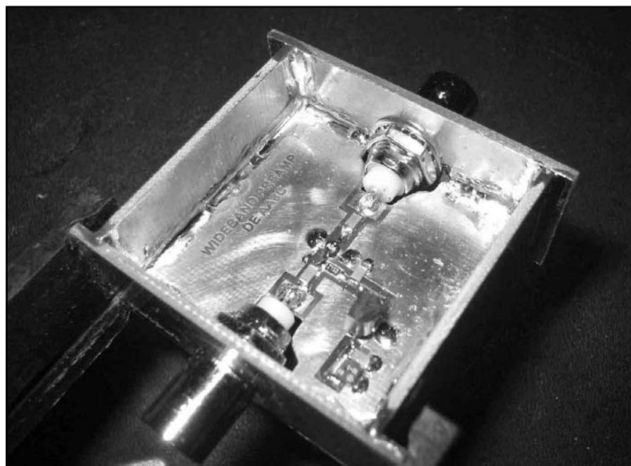
Fig 5—After all the panels are in place, carefully solder and fillet all seams before installing D1 and the feedthrough filter. Solder the BNC center pins after completing the assembly of the enclosure sides to be sure of adequate stress relief for the connections.
