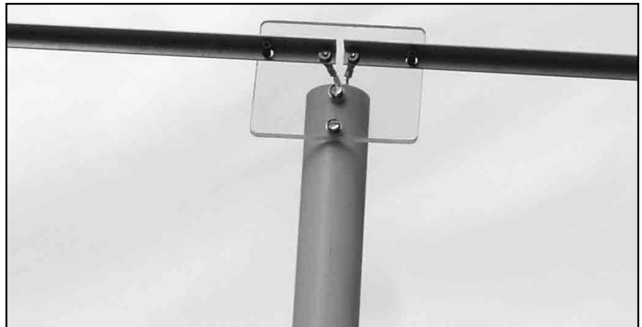
Photo C—The same assembly as in Photo B, but with an L-stock element—the outer support posts pass through holes in the element.
