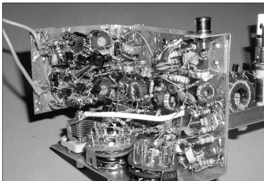
Fig 10—The RF/IF board is mounted outside the minibox on an L-shaped aluminum bracket attached to one end of the oscillator minibox.
