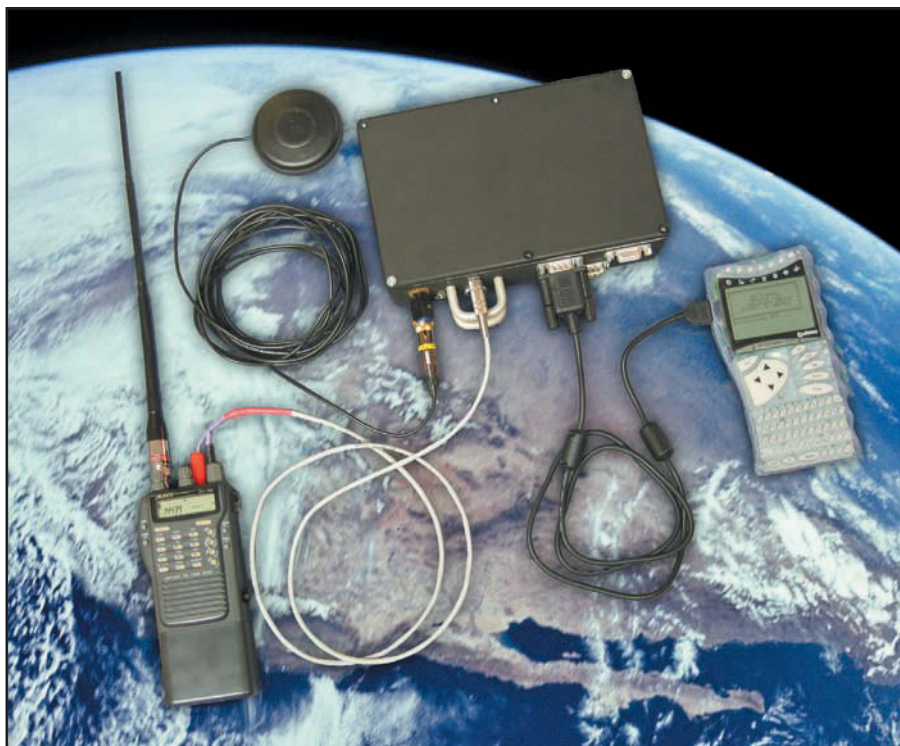
Fig 1—The complete Messaging BXTracker station. Teaming up with the VHF transceiver is a round magnetic active (pre-amplified) GPS antenna, the BXTracker and a Cybiko hand-held "pda" employed as a terminal. A Palm Pilot or Pocket PC can also be used as a terminal. The terminal is not required for normal or non-messaging use. Background Apollo 16 photo, courtesy NASA and the NSSDC.
