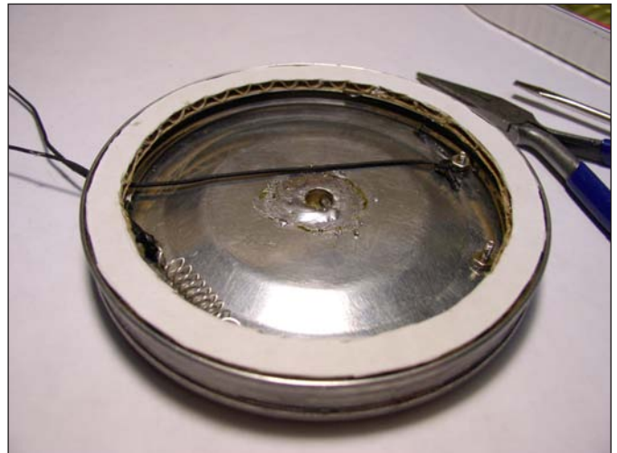
Fig 14 —A ½-inch-wide cardboard ring glued inside the dial drum rests on the narrow inner ring.
