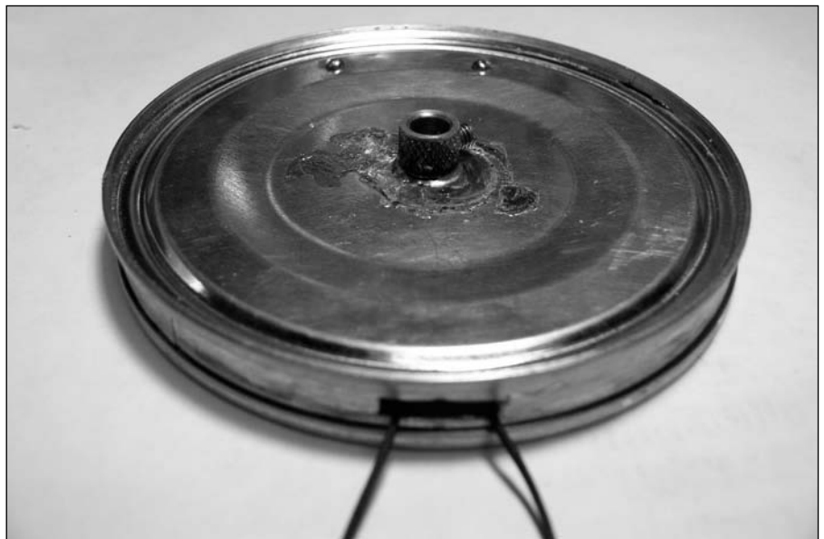
Fig 12—The position of the brass fitting soldered to the bottom of the dial-drive drum. A \frac{1}{2} -inch-long cutout in the cylinder completes the drum.
