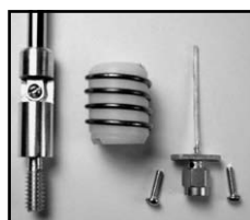
Fig 10— Disassembled matching network parts; radiator mount, coil, wire capacitor attached to SMA connector.
