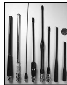
Fig 15—The hand-held antennas used for measurement comparisons to the homebrew half-wave antennas for 2 meters and 70 cm. In order from the left—Larson telescoping half-wave, AEA telescoping half-wave, Pryme quarter wave whip, Standard dual band for C510A, Larsen 2M, Larsen 70cm, Icom dual band for IC-Q7A, Standard dual band for C528A.
