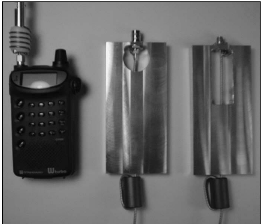
Fig 7—hand-held simulators used to measure the impedances and SWRs of hand-held antennas with either a BNC or SMA connectors.
