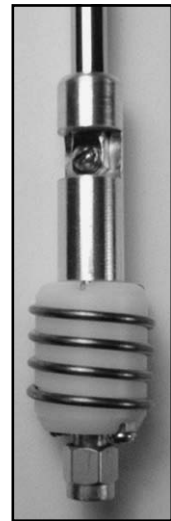
Fig 9—Matching network for 2-meter end-fed half-wave, telescoping element version.
