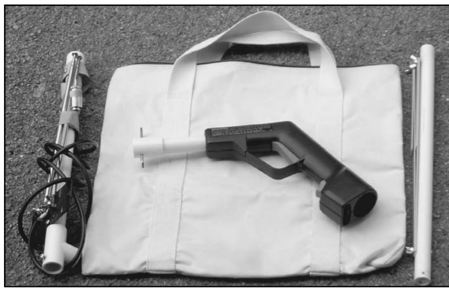
Fig 4—The demonstration Yagi broken into pieces for storage and transport.
