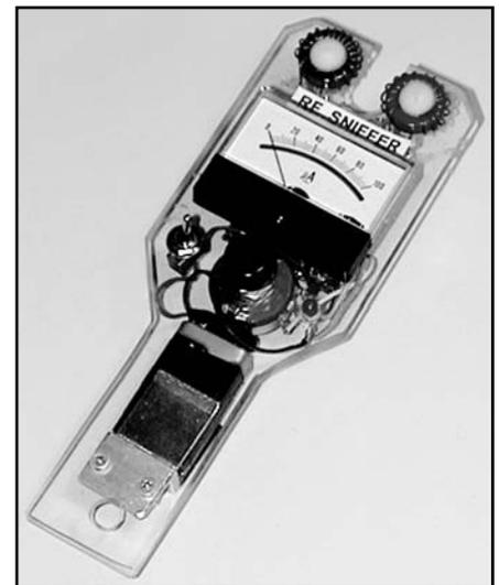
Fig 2—Voltage-canceling probe.
