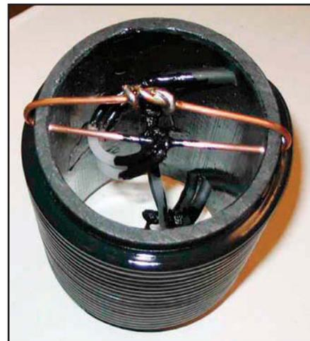
Fig 2—An end view photo of W6SQZ's trap.
