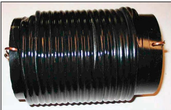
Fig 1—A side view photo of W6SQZ's trap.
