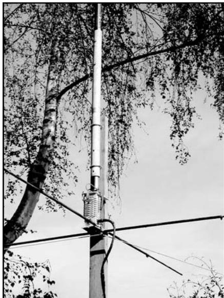
Fig 4—Base coil and radial elements.
