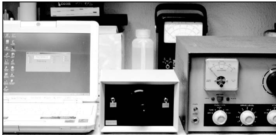
Fig 8—The VFO hard at work with the DX-60B (right). The notebook computer controlling the VFO is at left.
