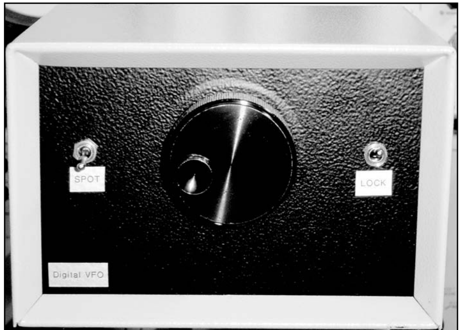
Fig 4—A front view of the VFO. The spot switch (S2) is at left and the lock switch (S3) is at right.
