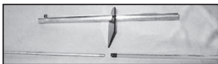
Figure 5 — The capacitor pieces are laid out ready for assembly. The plastic spacer is on the outer-sleeve tubing and will also attach to the main antenna-element tubing.
