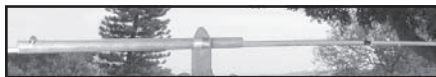
Figure 6 — In this case the capacitor is set for minimum capacitance, with the outer sleeve pulled back as far as possible.
