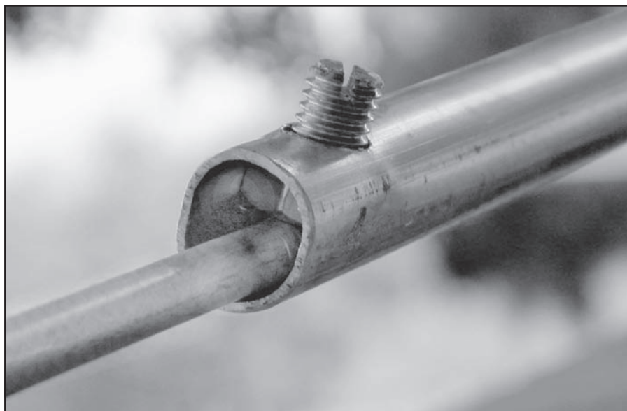
Figure 4 — This photo is a close-up view of the sliding coaxial capacitor.
