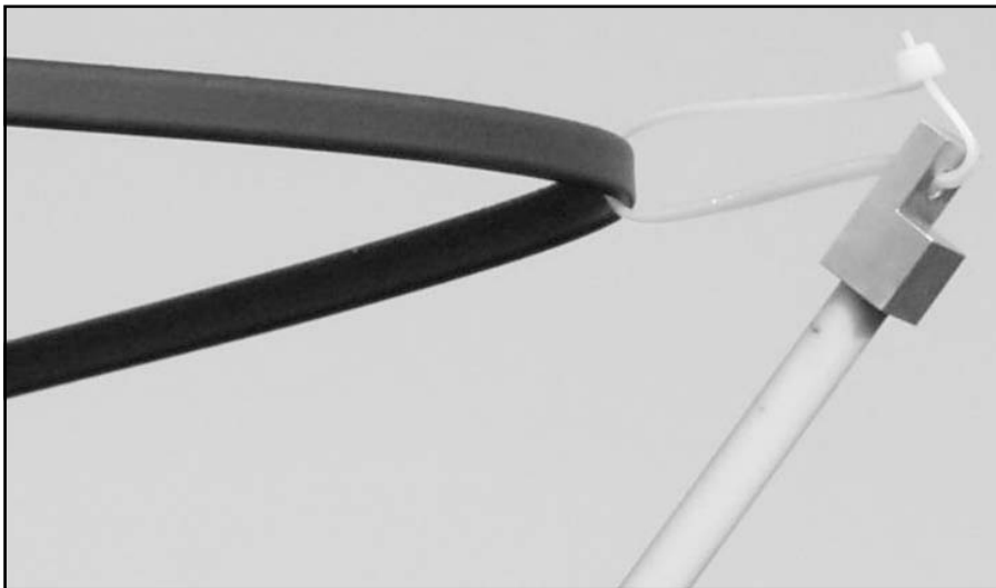
Figure 7 — This photograph shows the connection of the resonant cable loop to the end of the strut.
