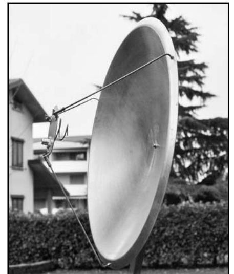
Figure 9 — The complete 60 cm disk antenna.
