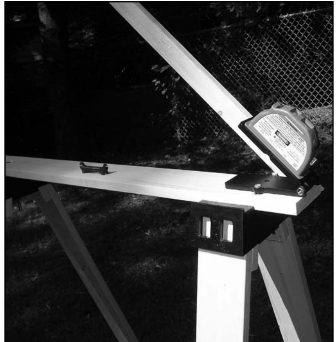
Figure 9 — Here a small laser level is attached to the sighting angle of the gizmo for possible nighttime measurements.
