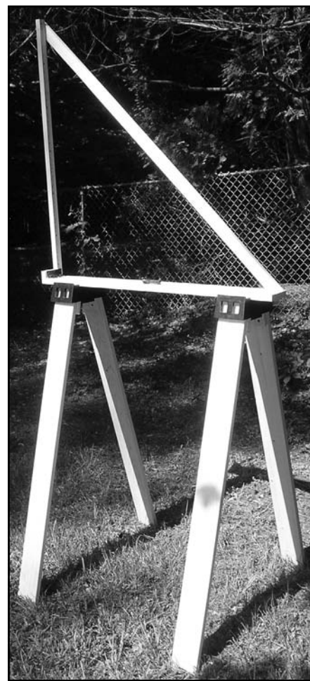
Figure 4 — This photo shows the gizmo opened ready to measure the height of a tree, tower or other object.
