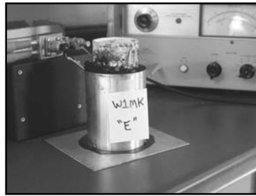
Figure 2 — Here is a photo of the test cell packed with a sample of soil under test, set up for a frequency sweep on the impedance meter.
