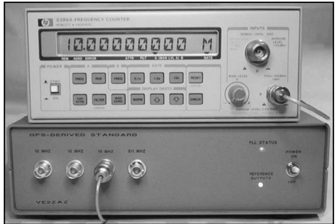
Photo B — This photo shows the GPS derived frequency standard connected to an HP frequency counter.
