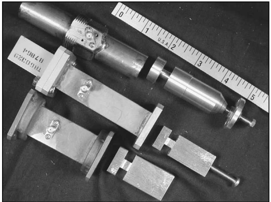
Figure 3 — Adjustable transitions for WR-90, WR-75 and circular waveguide.
