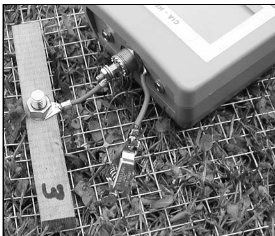
Figure 5 — This photo shows the details of how the impedance analyzer is connected to the probe and ground screen.
