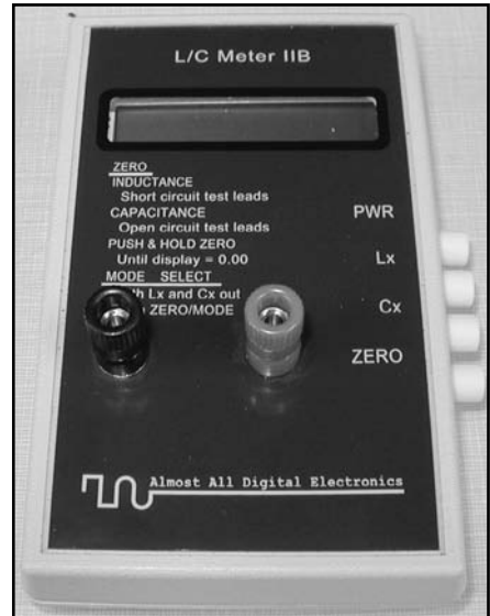
Figure A1 — I used this Almost All Digital Electronics L/C meter to measure the capacitance of the probes in air. By measuring the total capacitance of the probe and leads, and then measuring the parasitic capacitance, C_p , of the part of the probe above ground along with the connecting leads, I am able to calculate the capacitance of the probe alone, C_0 .
