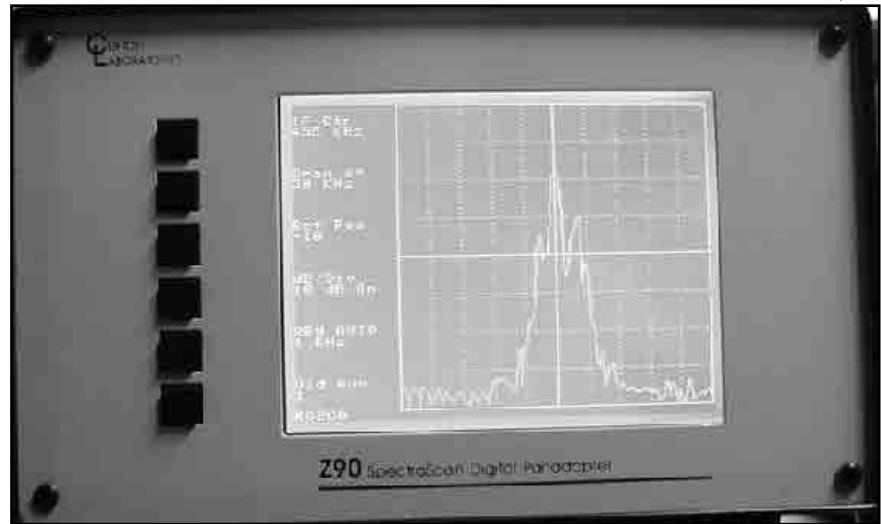
Figure 10 — Z90 Front panel showing soft keys and display graticule.
