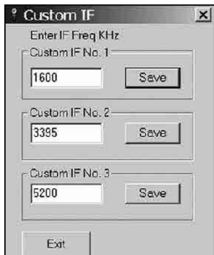
Figure 12 — Setting up custom intermediate frequencies via Z90-Control software.
