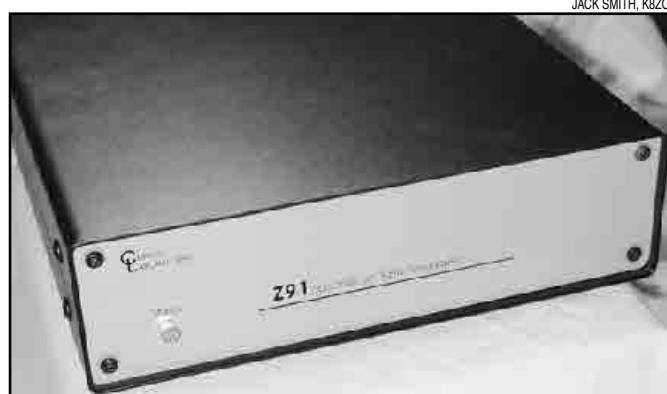
Figure 2 — The Z91 Digital Panadapter is similar but provides data only output for use with a compatible PC program.
