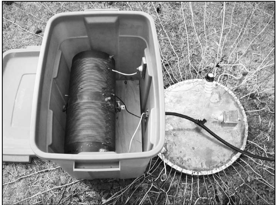
Photo A — Here is the loading coil and ground-radial connection in use at WD2XSH/20, Rudy Severns, N6LF.
