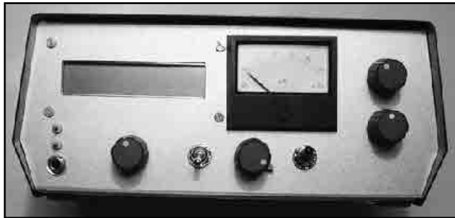
Figure 13 — This photo shows the front panel view of the transmitter, assembled in the box. From left to right/top to bottom: V_r +, V_r -, Key, DDS LCD Panel, DDS Frequency Tuning, Tune Switch, 5 A dc Meter, Output Power Adjustment, Band Switch 80/40 m, PA Tune, PA Loading.
