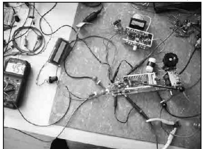
Figure 12 — This photo shows the prototype transmitter with the various sub units. To the left is the DDS module with LCD panel. At the top is the amplitude modulator, power control and keying circuitry. At the center of the photo is the RF unit with oversized heat sink and matching circuit components.
