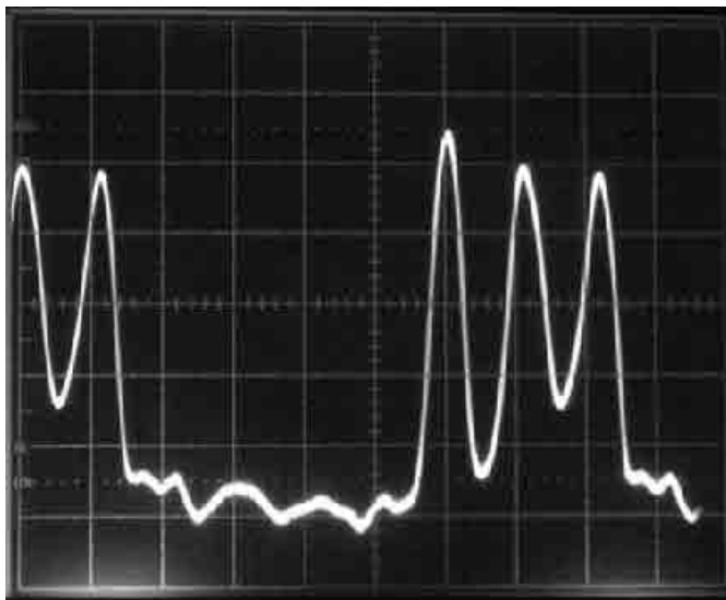
Figure 11 — Single drain waveform on 7 MHz with detuning; 10 V/division, 20 ns/division.
