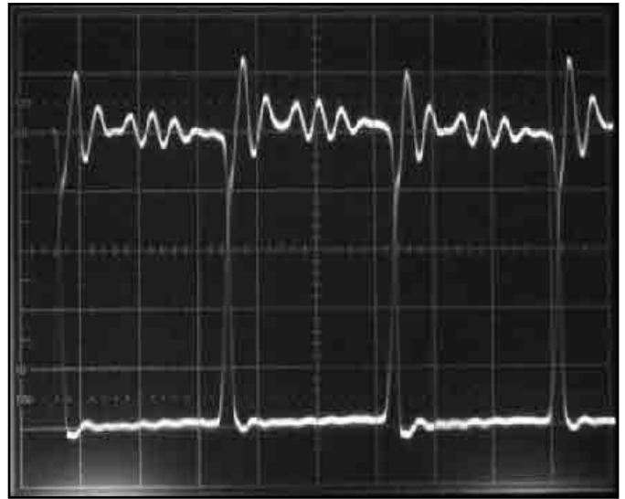
Figure 8 — This oscilloscope screen shows the same waveforms as Figure 7 but on 3.54 MHz; 5 V/division, 50 ns/division.
